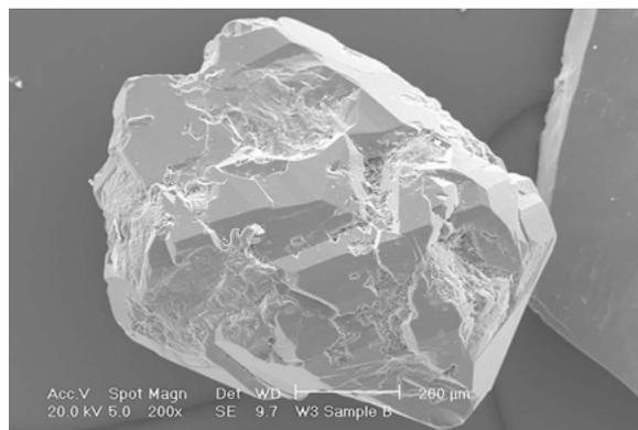
Source 1.6 Scanning electron microscope image of a river-worked quartz grain from the Hawkesbury River, New South Wales
